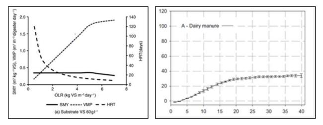
**Figure 1:** (a) Banks and Heaven (2013), showing a consistent BMP as represented by specific methane yield in the OLR range of 1-5; (b) Labatut et al (2011); biogas yield in mL against days
